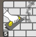
Apply the mix, using a putty patra or a rubber float. Firmly press the material into the groove.
