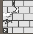
Make a V-groove on the crack, increasing its width on the surface to 5 mm using a handheld grout saw, cutter or putty patra. Make sure the groove is at least 5mm deep. Clean with water to remove any debris or loose particles, and allow to return to SSD condition.
