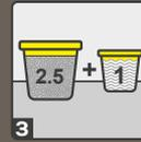
Gradually add 2.5 parts of weberwall crackbond to 1 part of clean water (by volume) and mix it to a lump-free, smooth workable paste using a suitable stirrer/low-speed drill mix/any other appropriate tool.
