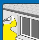
As with all structural concrete and cement mortars, good curing practice should be maintained. Water spray, wet hessian or a spray applied curing membrane should be used.
