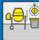
Add about 80 to 85 % water as per the mix design, to the running mixer and mix it for 1- 3 min.
