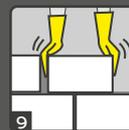
Firmly place the block with slight shear to ensure proper transfer and bonding.
