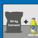
The recommended dosage is 200 ml per 50 kg of cement.
