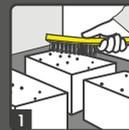
Always clean the surface before application to remove any loose particles or laitance.
