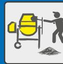
In a concrete mixer, add cement, aggregates and sand as per the mix design and mix the contents for 2- 3 min.
